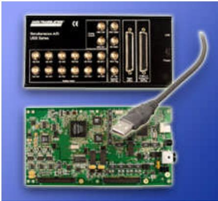
Data Translation application engineers proposed a unique answer that the manufacturer would not have thought of: Use two DT9836-12 high performance, isolated simultaneous data acquisition USB modules in tandem. The modules use the USB 2.0 bus, which is readily available on the notebook computer and provides the necessary throughput. At 225 kHz and 16-bit resolution
