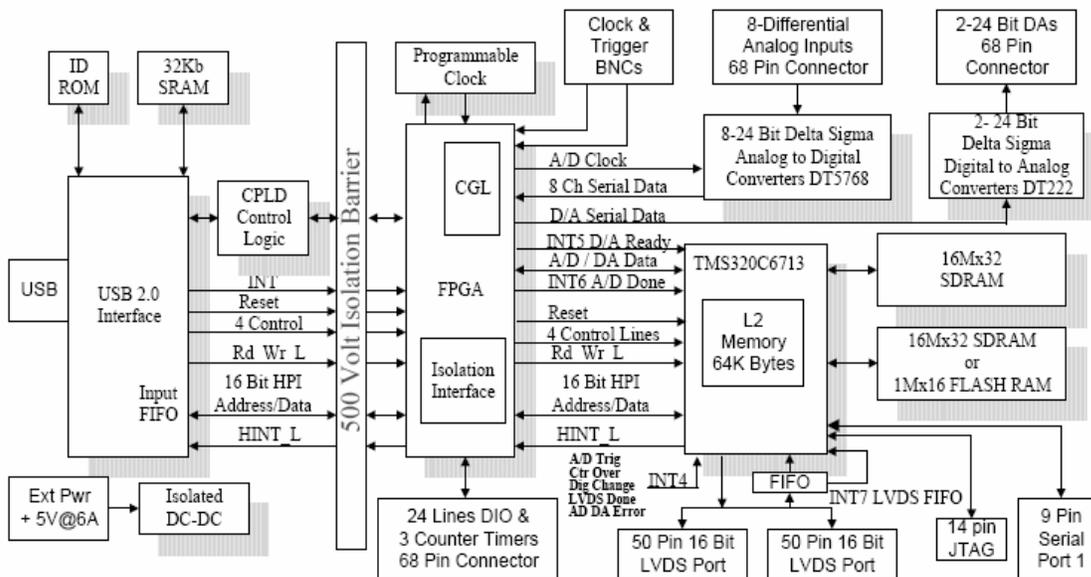
FIG. 1 – FUNCTIONAL BLOCK DIAGRAM OF DT9841
