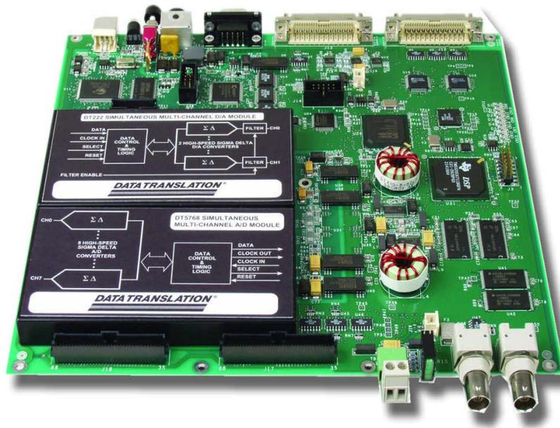
FIG. 2 – DT9841 FULCRUM II SERIES WITH TI C6713 FLOATING-POINT DSP
