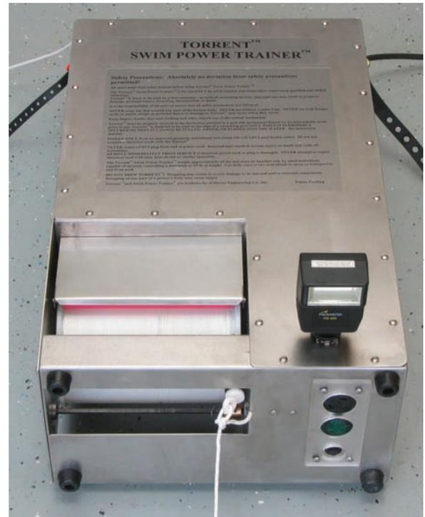
*The Torrent E-Rack is capable of measuring, graphing and displaying real-time swimmer data such as distance, time, speed, power, force, and maximum thrust*
