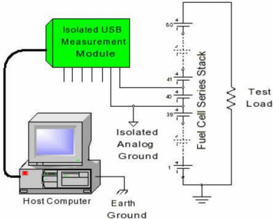
Figure 6: Isolation allows you to make floating-ground measurements instead of differential measurements referenced to ground.
