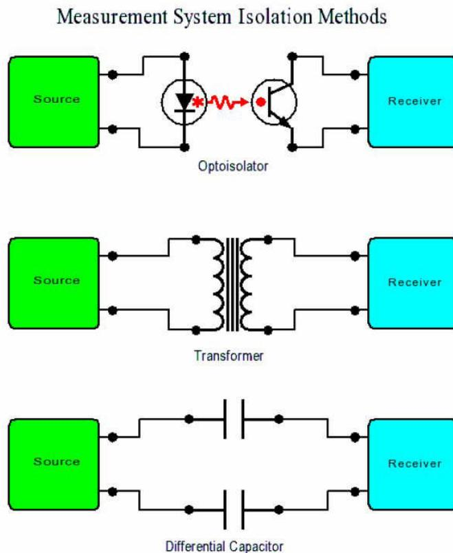
Figure 4: Three widely used isolation methods use non-electrical means to couple signals across an insulating gap: optoisolators use light; transformers use magnetic fields; and differential capacitive couplers use electric fields.
