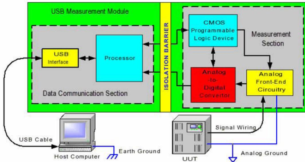
Figure 5: To isolate a USB measurement module, designers put an isolation barrier between the data communication and measurement sections, and add minimal processing power on the isolated side.
