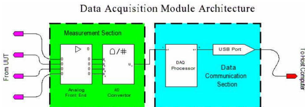
Figure 1: Data acquisition modules, whether built for PCI, USB or any other bus standard, have a communications section and a measurement section.
