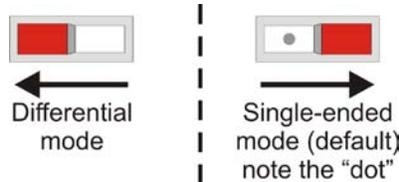
Figure 9. Channel input mode switch settings
