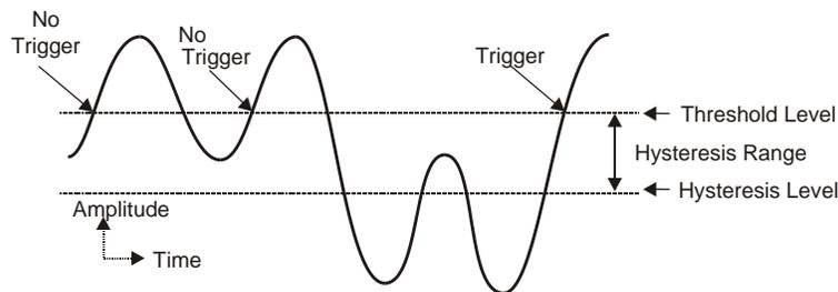
Figure 10. Hysteresis effect on a rising-edge trigger
