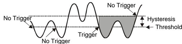
Figure 17: Falling slope, instantaneous duration, edge initialization
