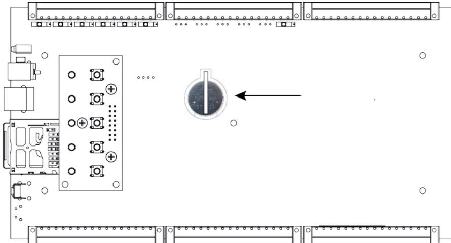
Figure 3. Location of battery compartment
