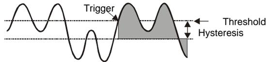
Figure 18: Rising slope, latched duration, edge initialization
