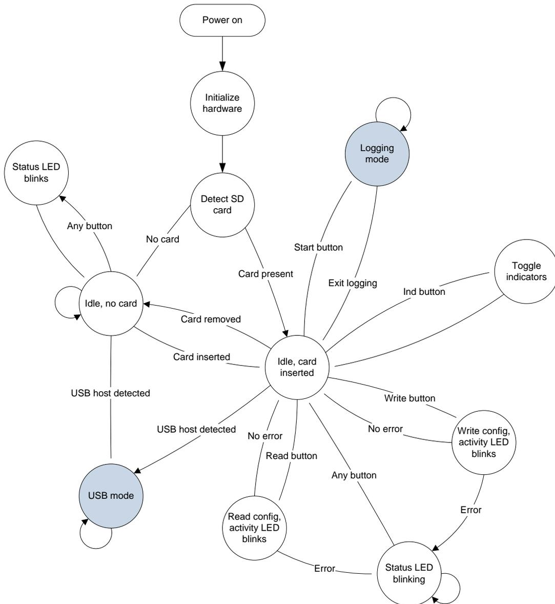
Figure 2. LGR-5320 Series USB mode/logging mode state diagram
