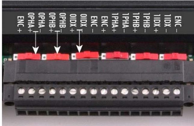
Figure 8. LGR-5327 and LGR-5329 counter channel input terminals and input mode switches
