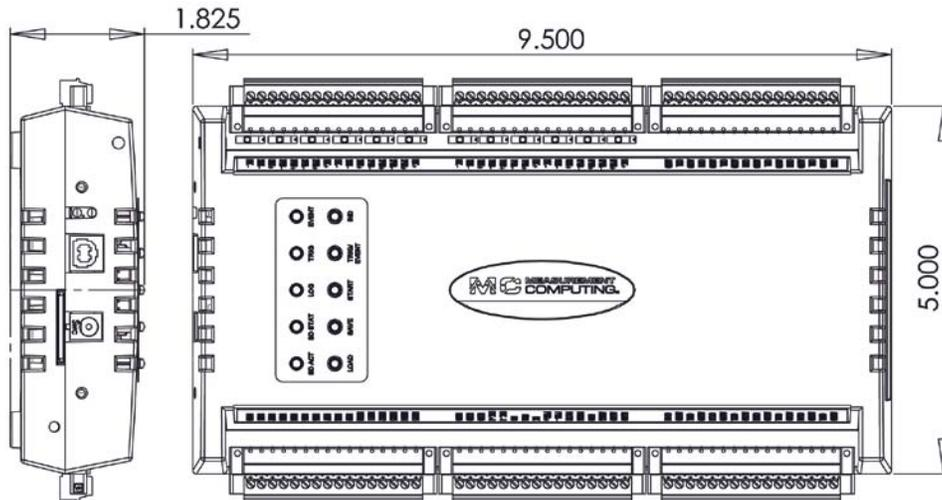
Figure 27. Housing dimensions
