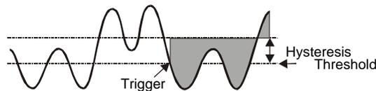
Figure 19: Falling slope, latched duration, edge initialization
