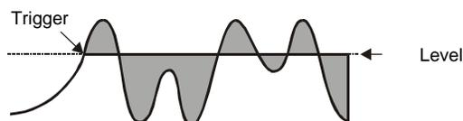
Figure 14. Above level initialization, latched duration
