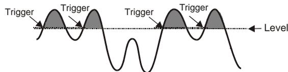
Figure 12. Above level initialization, instantaneous duration
