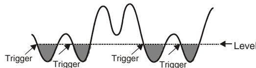
Figure 13. . Below level initialization, instantaneous duration
