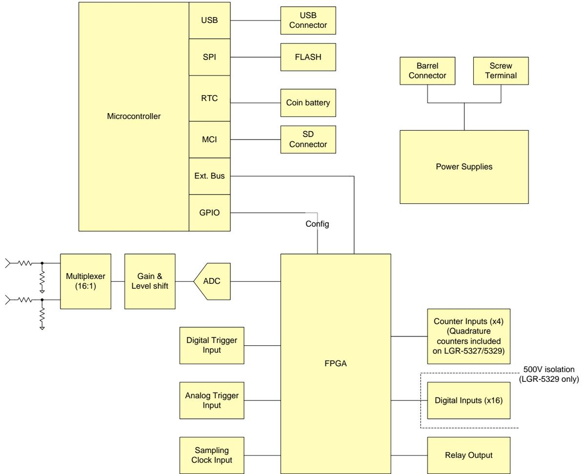
Figure 1. LGR-5320 Series functional block diagram
