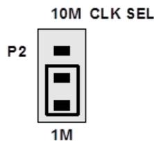
Figure 5. Clock frequency jumper
