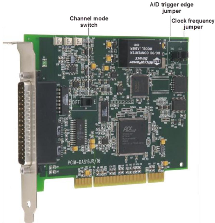
Figure 2. PCIM-DAS16JR/16 switch and jumper locations
