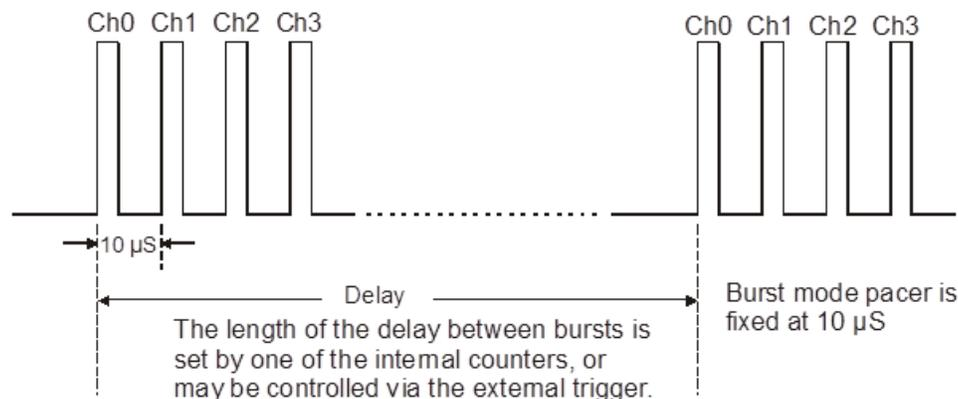
Figure 9. Burst mode timing
