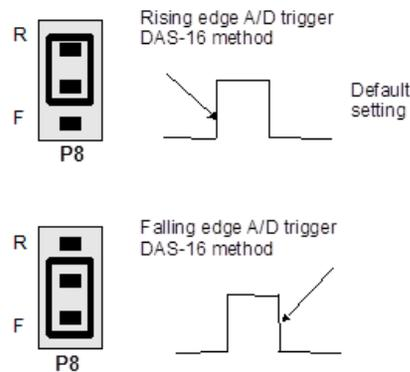
Figure 4. A/D trigger edge jumper
