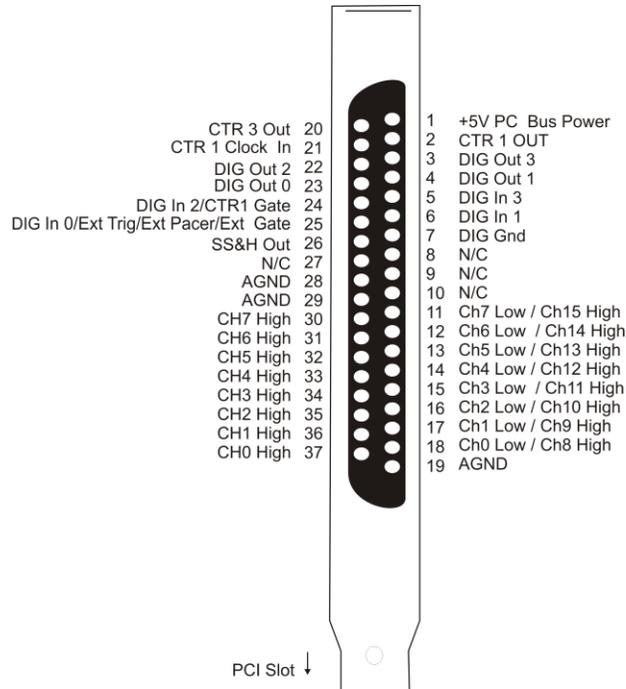
Figure 6. I/O connector pinout
