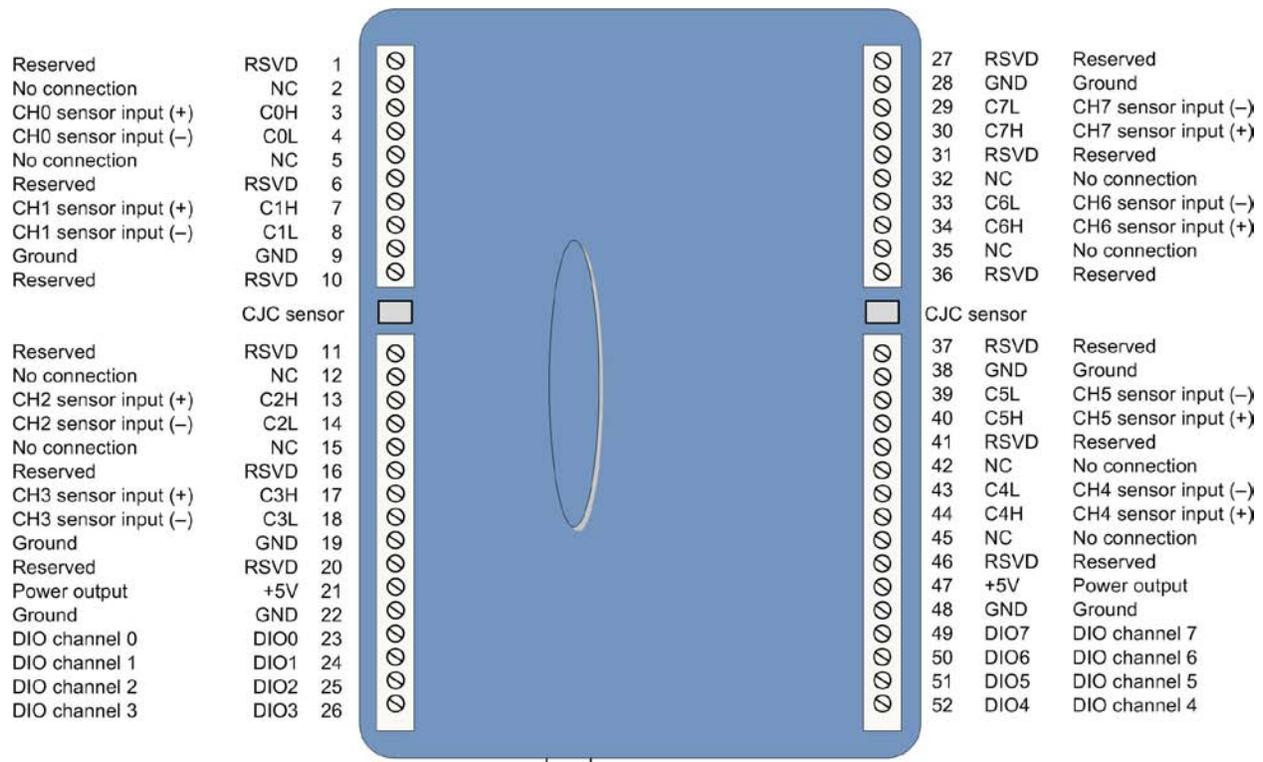
Figure 2. USB-5201 screw terminal pin numbers
