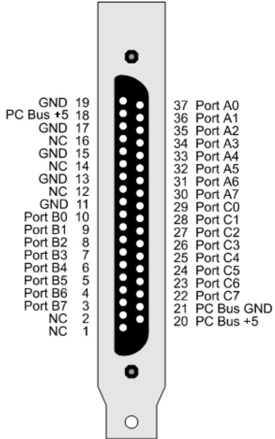
Figure 10. BP40-37 connector pinout
