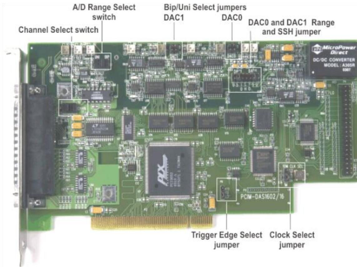
Figure 2. PCIM-DAS1602/16 switch and jumper locations
