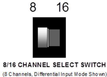
Figure 3. 8/16 Channel Select switch
