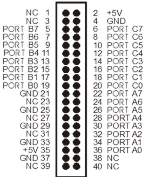
Figure 9. Digital connector pinout
