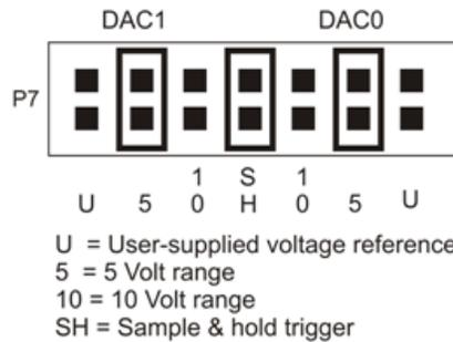
**D/A0 and D/A1 range jumper block**
