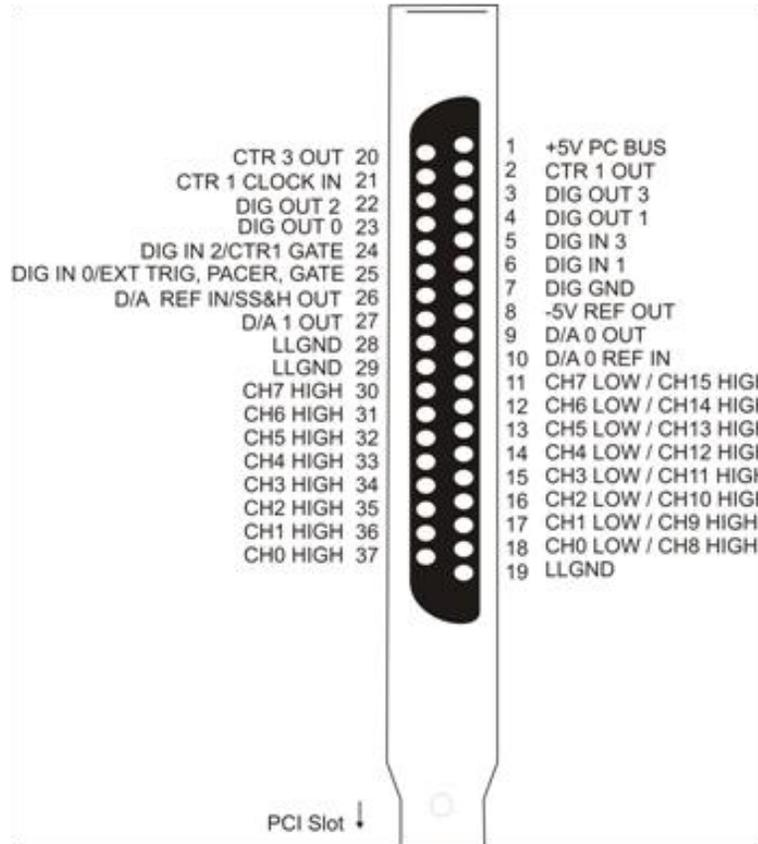
Figure 8. Analog connector pinout
