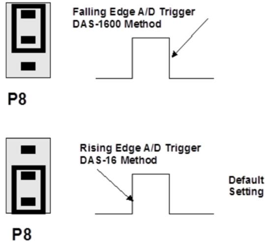
Figure 5. Trigger Edge Select jumper
