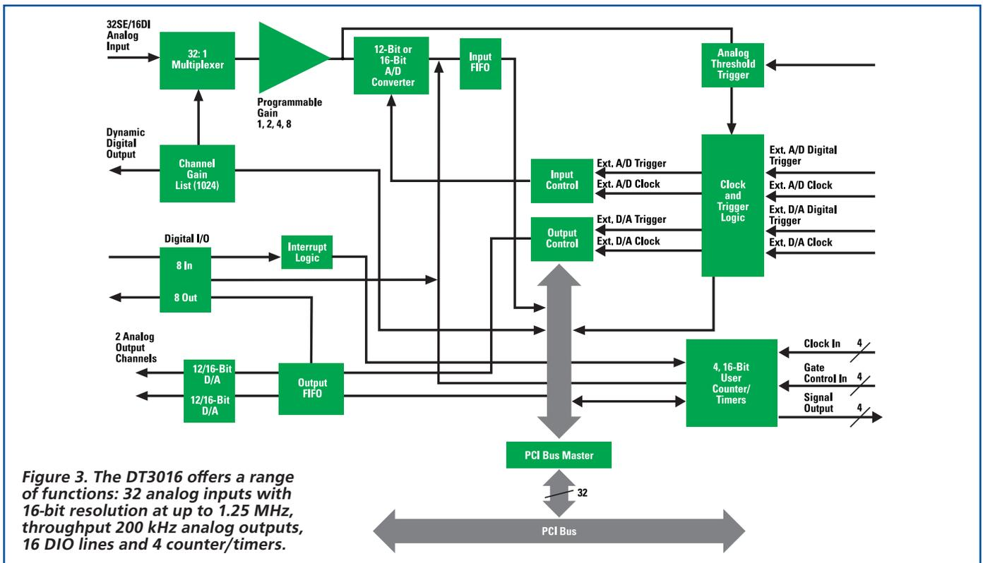
Figure 3. The DT3016 offers a range of functions: 32 analog inputs with 16-bit resolution at up to 1.25 MHz, throughput 200 kHz analog outputs, 16 DIO lines and 4 counter/timers.
