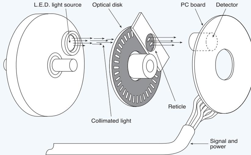
**Fig. 9.07.** The shutter is one of the most critical components of the encoder assembly. The sensor's resolution and accuracy hinge on the quality of the vendor's manufacturing and assembly processes.
