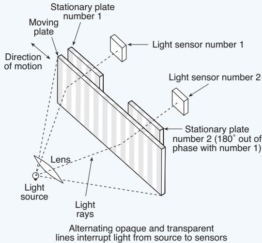
**Fig. 9.04.** Two-channel encoders provide step and direction vectors with an output signal that can be a sine wave, square wave, or a series of equally spaced pulses generated at regular intervals on the waveform.
