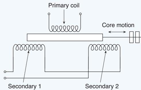
**Fig. 9.02.** LVDT sensors provide distance and direction information with extremely high accuracy. But a drawback for some installations is their relatively long length. The minimum length of the sensor is its body, and the core can extend only as far as the length of the body.
