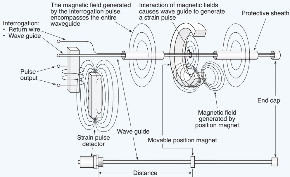
**Fig. 9.03.** Magnetostrictive position sensors have a high signal-to-noise ratio, shock and vibration resistance, and accuracy. They are rugged devices that deliver from 30 to 400 mV signals at their output terminals and require little or no additional signal conditioning. A possible disadvantage for some applications, however, is its wave-guide, which must be at least as long as the measured stroke.
