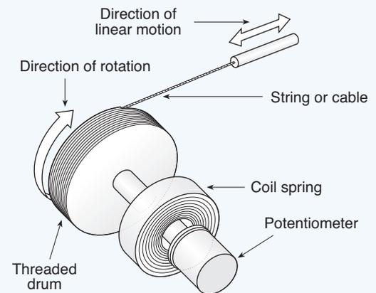
**Fig. 9.01.** String potentiometers occupy relatively little overall space in a machine installation or device under test. In some applications where a sensor cannot be mounted on the device being measured, the potentiometer may be conveniently located some distance from the test bed without sacrificing accuracy or repeatability.
