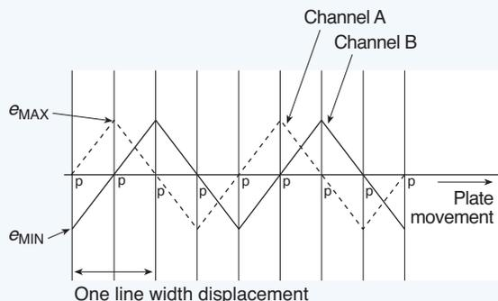
**Fig. 9.08.** The two light sensors in a dual channel linear position encoder are connected in a push-pull configuration and track one another, so equal changes in the input produce equal changes in the output.
