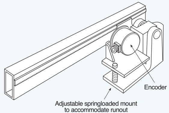
**Fig. 9.05.** A rack and pinion sensor assembly should have a flexible mount to compensate the combined runout error. In a machine application, the sensor should be protected from metal chips and other foreign objects to ensure measurement accuracy.
