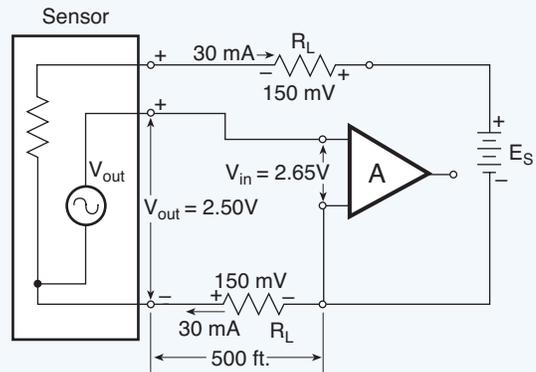
**Fig. 10.03.** The 150 mV dropped across  $R_L$  in the bottom ground return line arises from the 30 mA of current flowing in 5.2  $\Omega$  of lead wire resistance. The voltage adds to the sensor's 2.50V signal to yield 2.65V at the input to the signal-conditioning amplifier and produces a 6.6% error.
