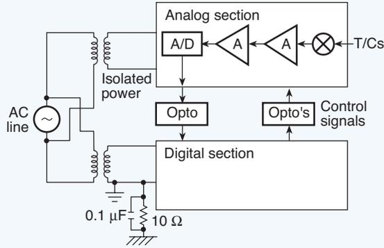
**Fig. 10.09.** Optical devices are the most widely used component for coupling signals across high-potential barriers and for low-level signals that are prone to the electrical noise typically coupled through different ground potentials.
