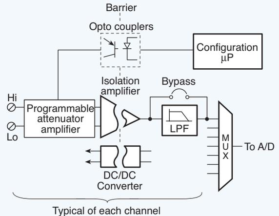
**Fig. 10.11** All three techniques of isolation are used in a multi-channel, programmable amplifier. Optical devices couple digital signals, capacitors couple analog signals, and the DC/DC converter supplies power to the isolated side.
