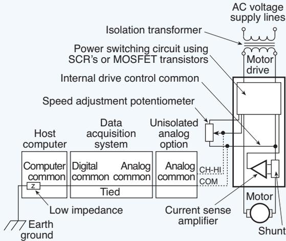
**Fig. 10.12.** Common-mode voltage is defined as the voltage between a signal and the localized common, which is usually earth ground. Common-mode voltages can be quite high, depending on the signal source. For example, a current sensing shunt in a DC motor drive might be expected to be at line-voltage potential, although the actual signal level is less than 50 mV across the shunt terminals. Measurement techniques for small signals at high common mode potentials call for isolation.
