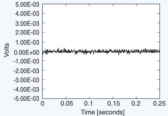
**Fig. 10.17.** The biggest improvement in reducing unwanted noise signals from the measured variable comes from differential-input amplifiers. It works so well because most of the noise on the high side duplicates the noise on the low side of the input and the algebraic sum of the two equal parts.
