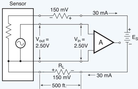
**Fig. 10.04.** A separate wire run from the sensor ground (or common terminal) bypasses the power supply ground wire voltage drop. The true output signal of the sensor ( $V_{out}$ ) reaches the amplifier input terminals because the input draws negligible current.
