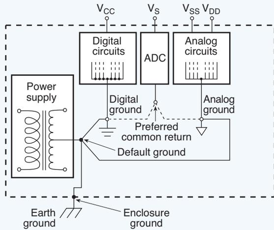
**Fig. 10.02.** Significant current fed to multiple circuits should have individual return paths to a common ground or negative terminal. This reduces the risk of voltage drops developing over long ground runs or lead wires that could become input (error) signals to other circuits.
