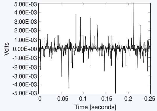
**Fig. 10.05.** Radiated noise spikes are easily picked up on non-twisted, non-parallel, unshielded lead wires connected to the single-ended amplifier input terminals, even when the inputs are shorted together.
