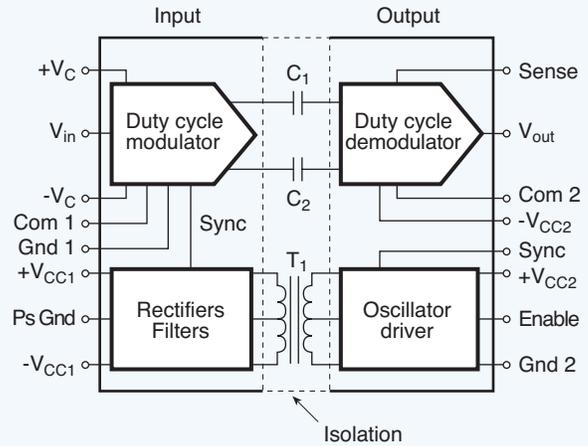
**Fig. 10.10.** Low-cost isolation amplifiers couple DC signals by modulating the signal, coupling its ac equivalent through a substrate capacitor connecting the stages, and then demodulating the signal to restore it to its original DC value.
