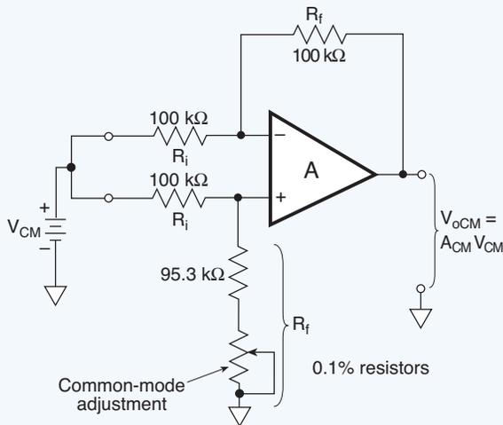
**Fig. 10.07.** Common-mode voltage is measured between the two input terminals and the common terminal. Because the two inputs must have identical voltages, they may be tied together and connected to one voltage source.
