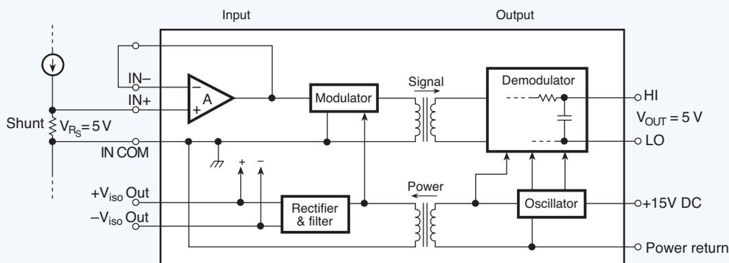
**Fig. 10.08.** This instrumentation amplifier with transformer coupling is typically used in an industrial process control loop and provides galvanic isolation in both input and output circuits. It can measure a  $\pm 5$  VDC signal riding on a common-mode voltage as high as 2000V.
