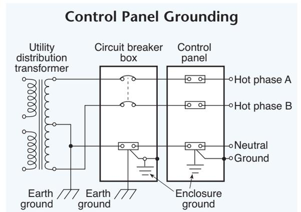
**Fig. 10.01.** Utility power transformers are typically grounded to earth ground near the transformer, and again at the input to the electrical junction box or first switching panel. The switching panel, in turn, may be connected to a rod driven into the earth to ensure that it too is at true ground potential.
